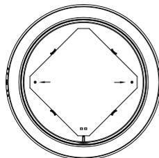
3. If there is no hot melt column in the lamp body or the hot melt column is not hot melt, this step will be adjusted without treatment. If the hot-melt column has been fused to fix the aluminum substrate, cut the hot-melt part of the hot-melt point with diagonal pliers.
