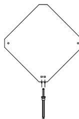
6. Take out two-cord cable (wire diameter 18-22AWG) and insert it into the plug-in terminal. Connect the external power supply for testing.
