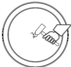
1. Power off, tap the central area of the diffusion plate with a pointed tool, and take out the cracked diffusion plate
