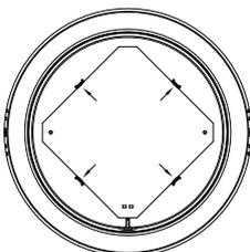
5. Press the buckle outwards, remove the aluminum substrate from the buckle, and remove the light source board.
