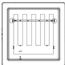
4. Press the buckle outwards, remove the aluminum substrate pressing strip from the bayonet, and remove the pressing strip. This step is only required for 24W panel light, other items are not required.
