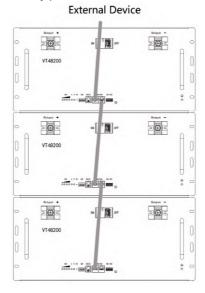
Figure 6-6 Connect RS485 Communication Cable
