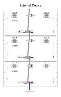
Figure 6-7 Connect the  $120\Omega$  Resistor
