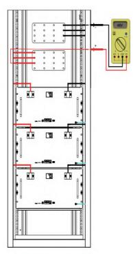
Figure 7-1 Check the Battery Voltage
