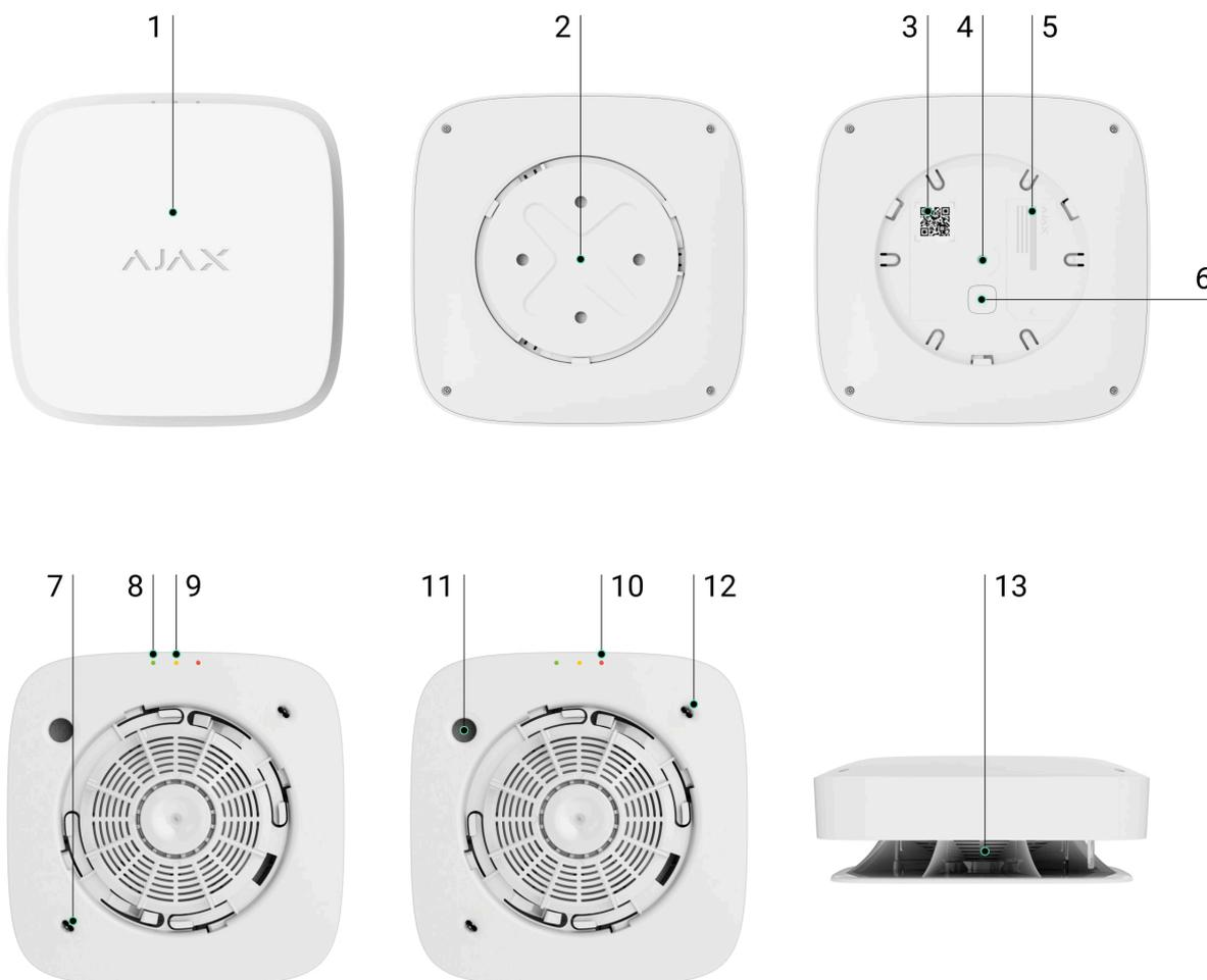
1. The front panel of the detector with a Test/Mute button. To activate the button, press the central part of the panel.
